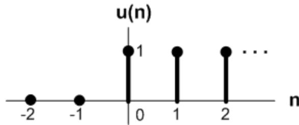
$$\begin{aligned} X(z) &= \sum_{n=0}^{\infty} u(n) z^{-n} = 1 + z^{-1} + z^{-2} + \dots \\ &= \frac{1}{1 - z^{-1}} , \text{ dimana } |z^{-1}| < 1 \rightarrow ROC : |z| > 1 \end{aligned}$$
