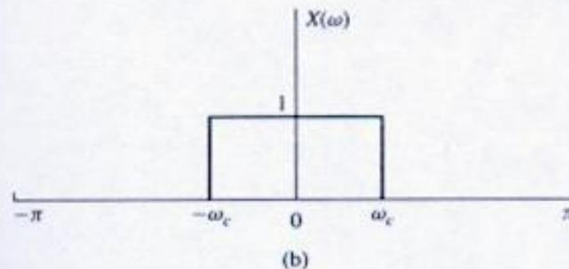
$$X(\omega) = \sum_{n=-\infty}^{\infty} x(n)e^{-j\omega n} \quad \longrightarrow \quad X_N(\omega) = \sum_{n=-N}^N \frac{\sin \omega_c n}{\pi n} e^{-j\omega n}$$
